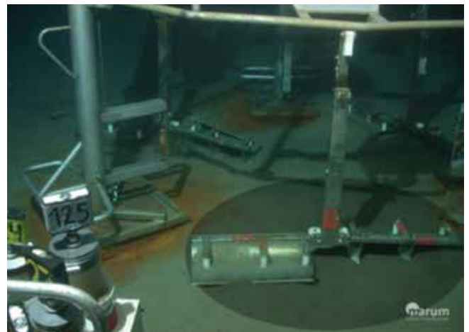
Figure 4: Autonomous Integrated Sediment Disturber deployed at the HAUSGARTEN site. In the lower left, push cores used for sampling by ROV are visible. The dark circle indicates one of three disturbed areas. Image courtesy MARUM/U.Bremen and T.Soltwedel, AWI.
